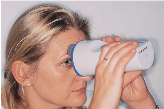
Fig. 10.7 The patient places the tonometer on his or her forehead and uses the fixation light to align it in the proper position. The head of the tonometer then automatically presses against the cornea, measures intraocular pressure, and retracts. Pressure is indicated in a digital display.
